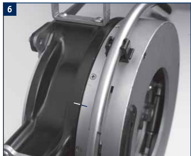
4 Make sure that the cutting unit is clear of the vice so that the pipe cutter can rotate freely.
