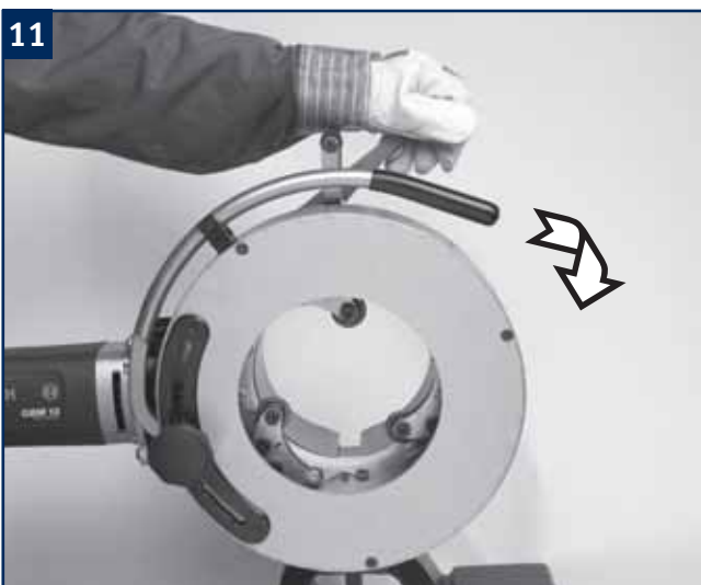
Push forward the hand lever for engagement of the cutting wheel unit to open the insert.
