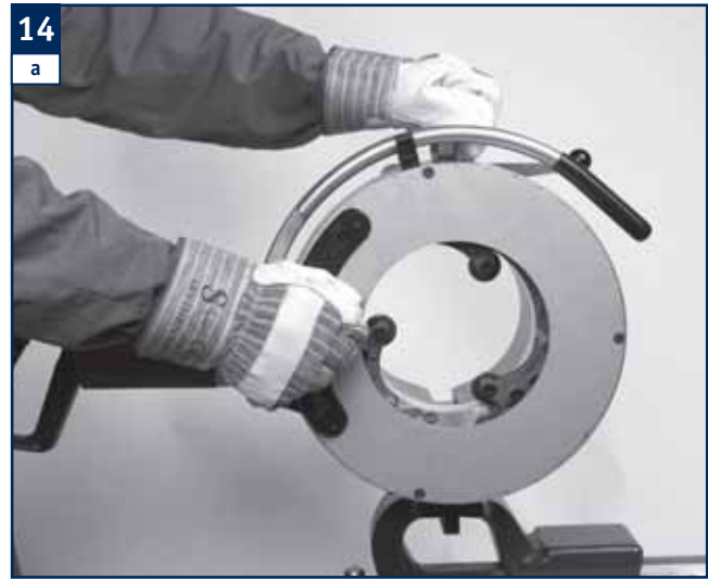
Use the hand lever to turn the cutting unit until the marking on the cutting unit is in line with the marking on the pipe cutter body.
