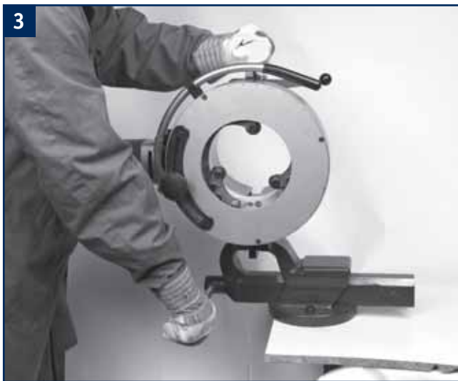
3 The pipe cutter is provided with a base plate for fixing in a vice.
