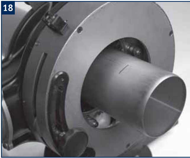
Position the pipe at the requested length.
