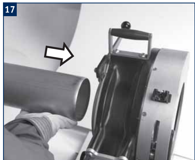
Insert the pipe from behind.
