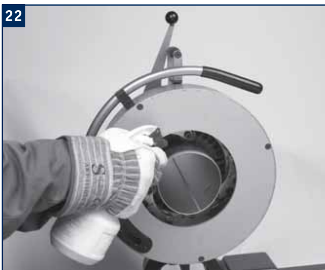
Add cutting lubricant at/on the cutting wheel.
