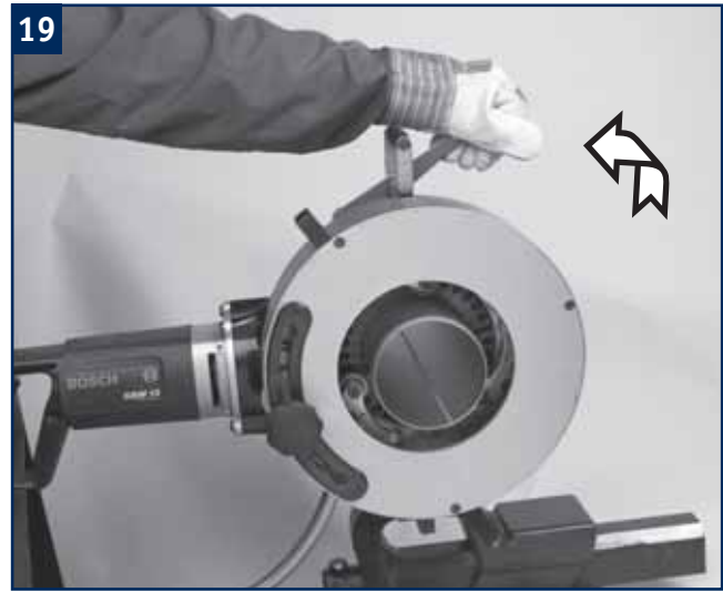
Pull back the hand lever to lock the engagement unit.
