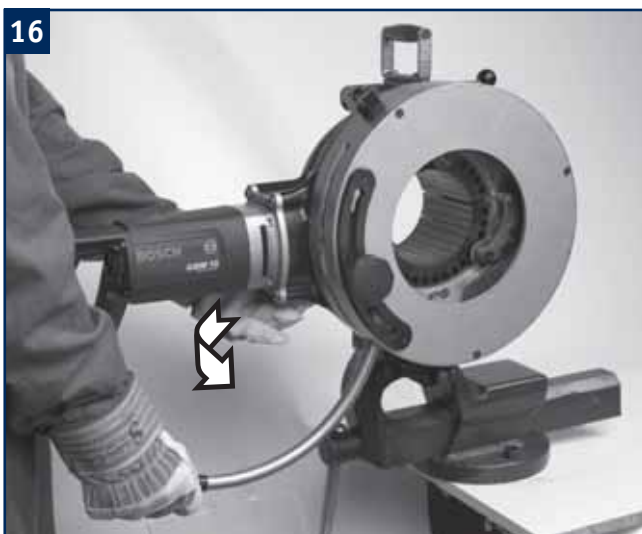
Push back the hand lever for opening the cutting unit.
