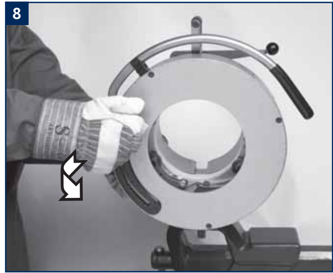
Pull out the hand lever to select the correct pipe dimension.
